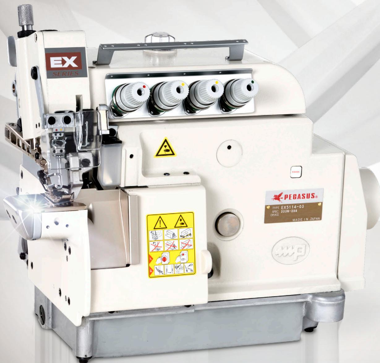
The EX series cylinder bed type machines most suitable for cylindrical goods.
