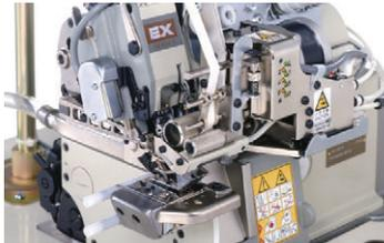
thread chain cutter cuts the elastic based on preset data. Thanks to this device, attaching elastic accurately and uniformly to tubular goods is easy.
