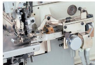
operator to concentrate on the sewing operation. In addition, if a presser foot that has a different fulcrum is used, the EX (T)5100 series will perform blindstitch hemming more steadily and beautifully.
