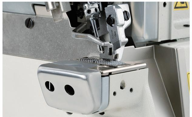
Thanks to the independently driven top feed mechanism, feeding efficiency has been increased dramatically. This feature responds to a wide variety of fabrics, including light to heavy weight fabrics.
